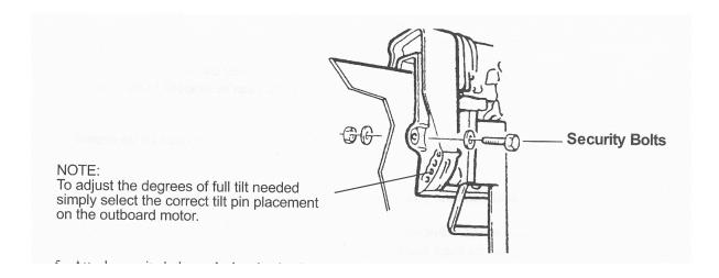
5. Attach security bolts to the bracket by drilling mounting holes into the bracket that match the size and location of the security bolt holes on the outboard bracket. Also use cable ties or other means to secure the clamp handles to prevent accidental loosening during operation.
