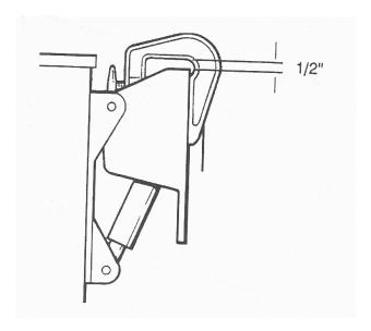
4. Before final installation, slowly run the bracket up to a full tilt to check for interference with the clamp bracket or the clamp handles. Reposition the motor as necessary.
