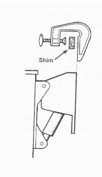
3. Leaving approximately a 1/2 inch space, tighten the clamps securely.
