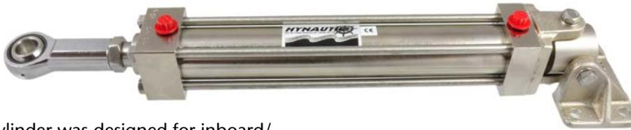
The **K-5-B** cylinder was designed for inboard/outboard boats requiring external cylinders of substantial size and strength. The **K-5-B** cylinders are nickel plated for aesthetics and protection against the elements. This cylinder does not include the wing plates or hardware required for mounting to the outdrive. Porting is through two through-hull 1/4" NPT ports located at the mounting end of the cylinder.
