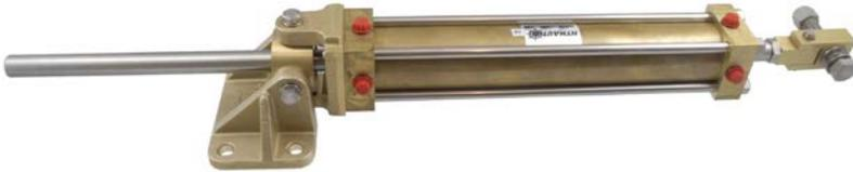
The K-9 cylinder is a double rod end, tie rod constructed hydraulic cylinder. This cylinder has a universal mount, which allows two planes of pivot freedom. This cylinder is equipped with a stainless steel ball joint. Porting is through two 1/4" ports at each end of the cylinder.
