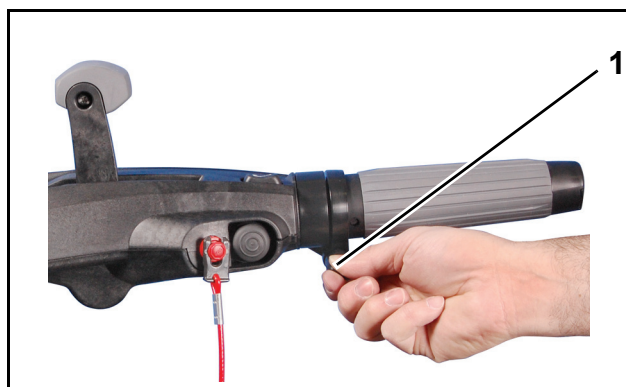
1. Throttle friction knob
