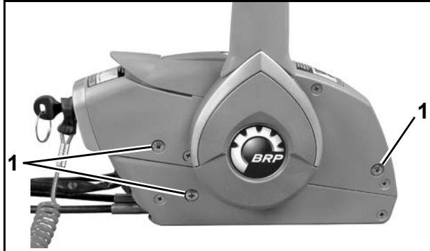
Port Mounting Configuration 1. Screws (3)
