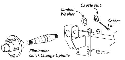
NOTE: Hub & Tire Carrier can be used with any trailer using a 5 lug 1750# UHI Hub, Quick change spindle can only be used with a 3500/3750# Eliminator Torsion Axle.
