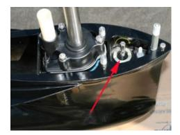
**2.5** The gearcase needs to be shifted into forward. Turn the shift rod (arrow) clockwise while turning the propshaft counter clockwise. You will feel the propshaft lock into position when the forward gear position is reached. The shift shaft will no longer be able to turn clockwise as well. In forward gear, when you turn the driveshaft clockwise; the propshaft will turn clockwise.
