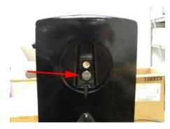
**1.5** Below the trim tab is bolt which must be removed. On newer models it will be 18mm. On older models it will be 9/16".
