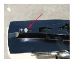
**2.4** Insert the trim tab bolt into the rearward of the two holes at the back of the SE206 unit (arrow).
