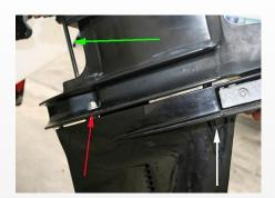
**2.8** Place flat washers on the two studs facing upward and hand tighten two nuts onto the threads (red arrow). Check to make sure that the shift rod is not bound up (green arrow). If the shift shaft is bound, slide the shift cable retainer (under engine cowling) back and forth slightly until the shafts align. Once everything is aligned, install washers and nuts on the two studs facing downward (white arrow) and tighten all four nuts in an alternating pattern. Torque the nuts to 50 lb-ft.
