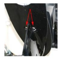
**1.7** Using a 5/8" socket, remove the two lower nuts (arrows). Use caution as these are the last two nuts holding the gearcase to the midsection. The unit may fall off if you are not holding it. Remove the unit and set it aside.
