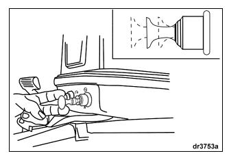
After installation, check for fuel leaks.
