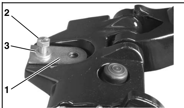
1. Shim plate 2. Steering arm screw 3. Washer 002398
