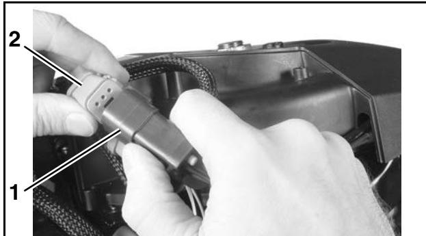
1. Tiller handle wiring harness 2. Engine wiring harness 002423
