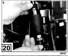
Install sleeve saved in the center of new pump body. Apply *Triple-Guard®* grease to O-ring on top fitting (a) saved, and to new pump cavity. Install fitting in pump. Torque fitting to 60-80 in. lbs. (7-9 N·m).
