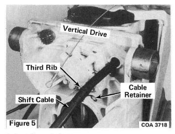
6. Install vertical drive as shown in your service manual or instruction sheet. Fasten cable retainer to intermediate housing using screw and lock washer. See Figures 6 and 7.
