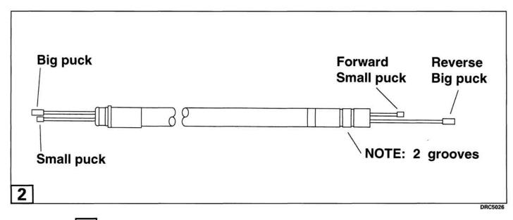
**2** Mechanical shift cables used on lower gearcases with anodes can be identified in two ways:
