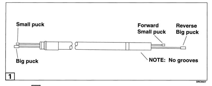
**1** Hydro-mechanical shift cables used on lower gearcases without anodes can be identified in two ways:
