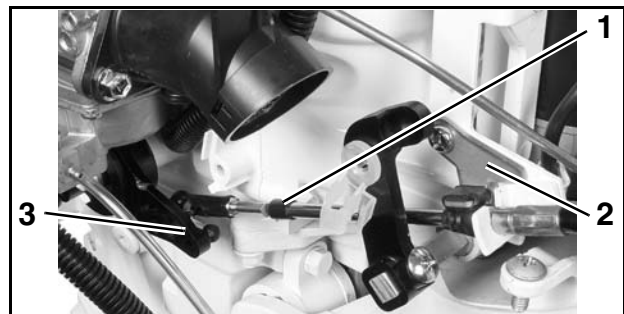
1. Throttle cable 2. Cable holder 3. Throttle drum
