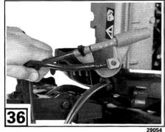
A Place rubber boot over starter solenoid top terminal stud. Coat remaining starter solenoid terminal studs with *Black Neoprene Dip.*
