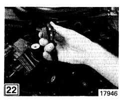
18 19 V8 MODELS Move starboard power pack aside to clear flywheel. Raise electrical bracket and locate single-wire connector (a) from black/yellow wire under bracket. Remove and discard tie strap securing switch cable to timer base wires. Separate plug and receptacle. Remove black wire terminal (B) from lower starboard crankcase screw. Remove terminal from screw and reinstall screw. Replacement switch cable black wire will be relocated to electrical bracket screw.
