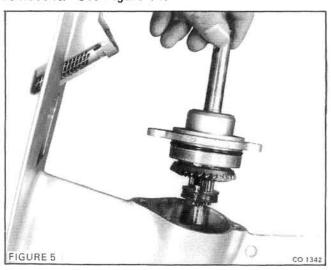
15. Remove forward gear and bearing by using propeller shaft or a bar of same diameter and rotate the forward gear and bearing around pinion gear to remove. See Figure 12.
