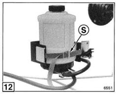
9. The fuel line fittings may be repositioned if necessary for improved fuel line routing. Loosen retaining ring with strap wrench or in vise, turn pump assembly (i) to desired location, and retighten retaining ring to fix pump position and seal tank.
