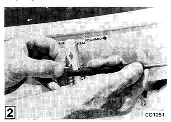
Install Adapter Kit to port and starboard side of engine.
