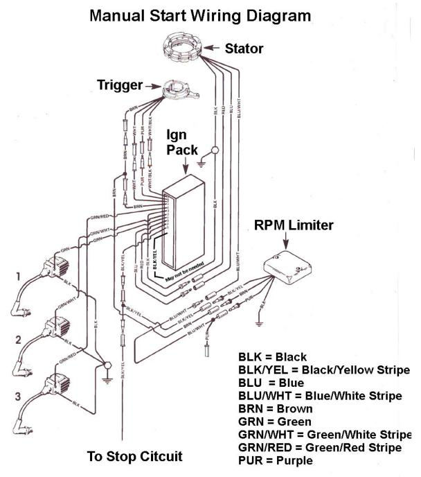
NOTE: Some engines use GRN/RED for #1, GRN/WHT for #2 and GRN for #3 cylinder. If engine backfires or seems to be out of time, index the flywheel and verify timing on each cylinder. Adjust the Green wires to reflect the correct firing order for your engine.
