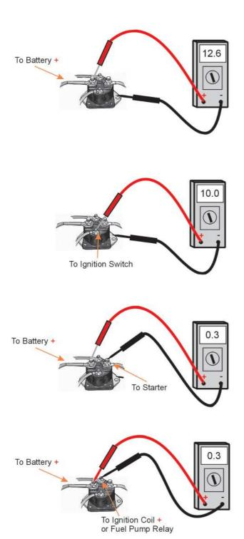
**Step 1:** Check the voltage on the battery side of the solenoid as shown on the left. The reading should be the same as the battery reading (12.6V = Full Charged Battery).
