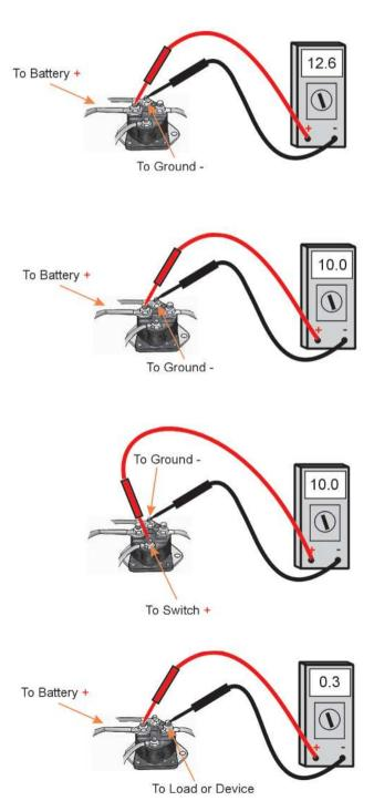
**Step 1:** Check the voltage on the battery side of the solenoid as shown on the left. The reading should be the same as the battery reading (12.6V = Full Charged Battery).
