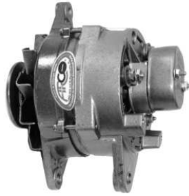
Brush Cover Installed
