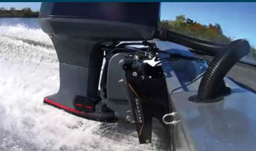
SeaStar HD Jackplate with a 350HP engine.
