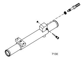
P/N 861156A04 - Fuel Pump/Cooler Kit, W/ Drain - has cooler P/N 807950, which has an integral water drain port and has a fuel line retaining bolt that is parallel to the fuel line to attach the fuel line to the fuel cooler outlet
