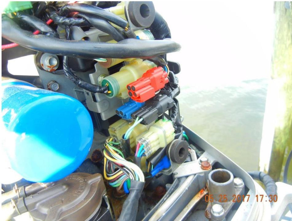
Once connected, turn on the key switch and observe the number of blinks on the check engine (MIL) light. The blinks will repeat until you turn off the key.
